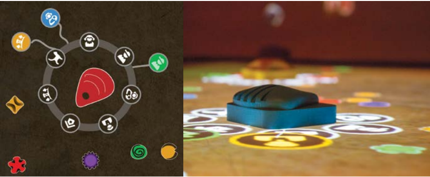
Figure 4: A menu of icons appears when a tangible shell is placed on the table and a story can be created by dragging beads onto the icons displayed around the shell (left); the shells were designed in 3D modeling software and fabricated using a 3D printer (right).
